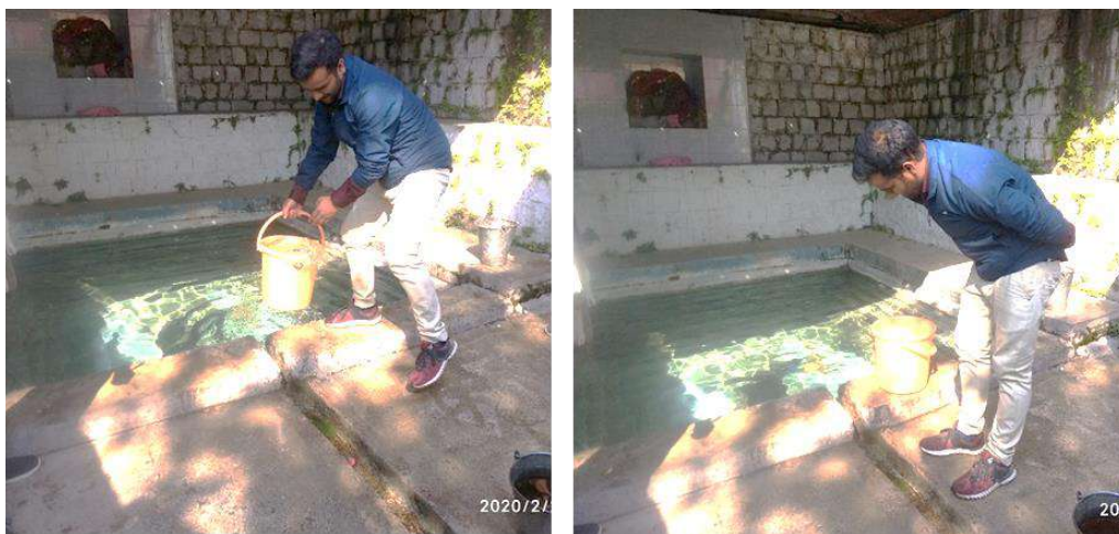
Fig. 5.5. Discharge measurement of a Seep type spring.
