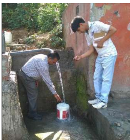
Fig. 5.4 Discharge measurement of a Free flow spring.
